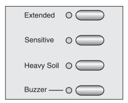
■ Use the corresponding button to select any desired extras. When an extra is selected, the matching indicator light comes on.
